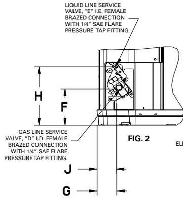
ELECTRICAL AND REFRIGERANT COMPONENT CLEARANCES PER PREVAILING CODES.
