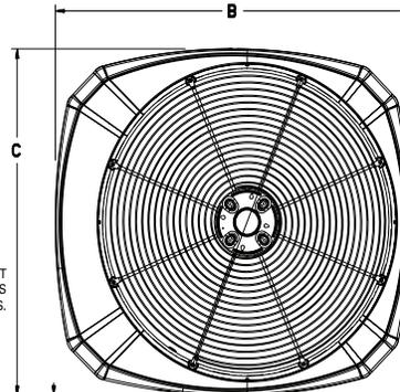
TOP DISCHARGE AREA SHOULD BE UNRESTRICTED FOR AT LEAST 1524 (5 FEET) ABOVE UNIT. UNIT SHOULD BE PLACED SO ROOF RUN-OFF WATER DOES NOT POUR DIRECTLY ON UNIT, AND SHOULD BE AT LEAST 305 (12") FROM WALL AND ALL SURROUNDING SHRUBBERY ON TWO SIDES. OTHER TWO SIDES UNRESTRICTED
