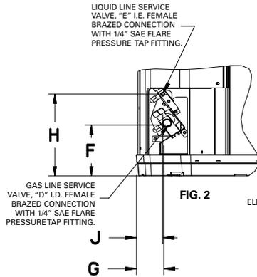
ELECTRICAL AND REFRIGERANT COMPONENT CLEARANCES PER PREVAILING CODES.
