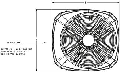
TOP DISCHARGE AREA SHOULD BE UNRESTRICTED FOR AT LEAST 1524 (5 FEET) ABOVE UNIT. UNIT SHOULD BE PLACED SO ROOF RUN-OFF WATER DOES NOT POUR DIRECTLY ON UNIT. AND SHOULD BE AT LEAST 305 (12") FROM WALL AND ALL SURROUNDING SHUBBERTY ON TWO SIDES. OTHER TWO SIDES UNRESTRICTED.
