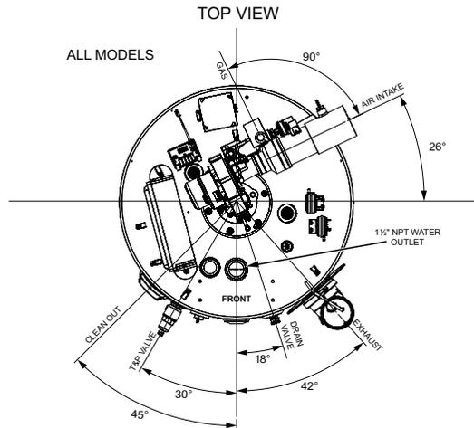
\* Center line of water outlet on top of the water heaters is approximately 7 inches from the front edge of the water heater
