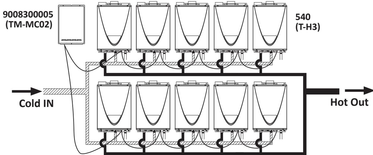
An individual cut-off switch is recommended for each unit in a Multi-Unit System for the purpose of maintenance.
