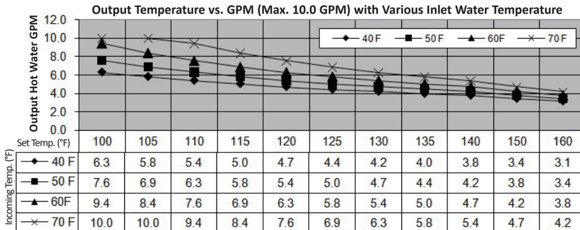
\*When the set temperature is 130 °F (55 °C) or higher, maximum flow rate is limited to 8.0 GPM.
