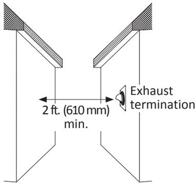
Exhaust and/or direct-vent sidewall terminations should be at least 2 ft. (610 mm) away from an opposite surface/wall. Do not place the termination directly in front of an opening into a building.
