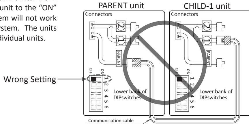
**CASE 2: Wrong connections between the "PARENT" unit and the "CHILD-1" unit**
