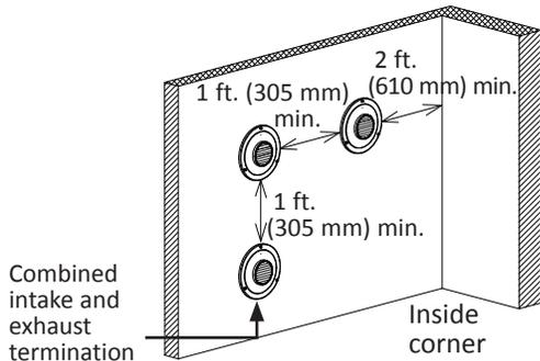
For multiple-unit, direct-vent sidewall terminations that combine the intake and exhaust into a single penetration, space each direct-vent termination at least 1 ft. (305 mm) away from each other, no matter the orientation. A direct-vent termination must also be at least 2 ft. (610 mm) away from an inside corner. (If the adjacent wall is less than 2 ft. (610 mm) of length, the minimum required distance away from the inside corner will be equal to the length of that adjacent wall.)
