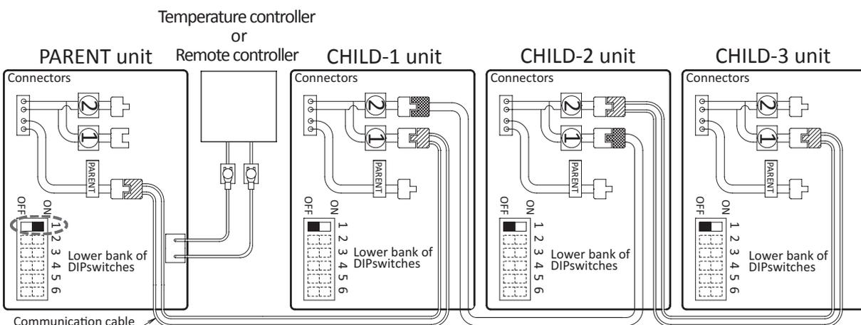
**NOTE:** The dark squares indicate the direction the DIPswitches should be set to.
