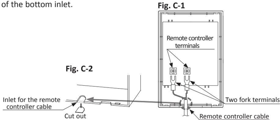
**<How to connect the remote controller to the water heater>**
