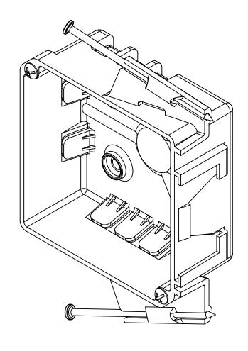
NOTES: 1.) BOX MATERIAL:POLYCARBONATE, NAIL MATERIAL: PLATED CARBON STEEL, SCREW MATERIAL: ZINC PLATED STEEL 2.) UL LISTED WITH 2 HOUR FIRE RATING FOR WALL
