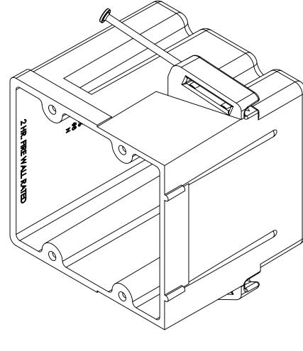
NOTES: 1.) BOX MATERIAL: FIBERGLASS REINFORCED POLYESTER, NAIL MATERIAL: PLATED CARBON STEEL, CLAMP MATERIAL: GALVANIZED STEEL, CLAMP SCREW MATERIAL: ZINC PLATED STEEL 2.) UL LISTED WITH 2 HOUR FIRE RATING FOR WALL
