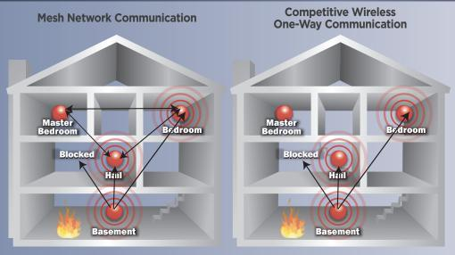
BRK Wireless Interconnect alarms operate on a "mesh network"; a 2-way communication format that sends, receives and then re-sends the alarm signals. If the initiating alarm signal is blocked from reaching one of the alarms, the mesh network communication reroutes and re-sends the signal via the other alarms as shown in the illustration. With competitive one-way wireless communication, only the initiating alarm sends a signal which may never be received, leaving the blocked alarm deadly silent.
