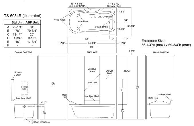
Sump Dimensions: 50" long x 21-1/4" wide x 15-3/4" deep / Sump Capacity: 54 gal. (unoccupied - to overflow)
