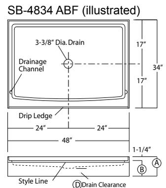
**Illustration 1b - Center Drain, Unit Dimension & Alcove Framing Guidelines (dimensional tolerance +0 / -3/8")**
