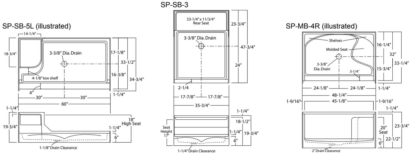
**Illustration 1c - Center Drain, Unit Dimension & Alcove Framing Guidelines (dimensional tolerance +0 / -3/8")**
