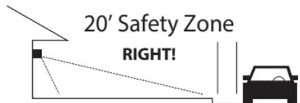
7. Make sure heat from lights is not triggering sensor. Make sure sensor is *below* and as far as possible from lights.
