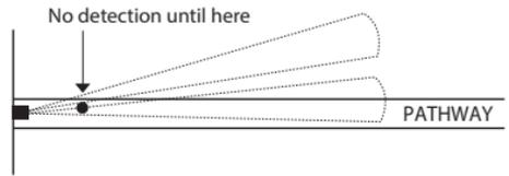
**Solution:** "Micro Adjust" sensor by moving sideways 1/4". This may move the zones to allow earlier detection.
