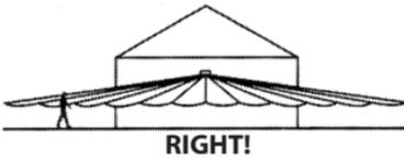
2. Check that the sensor is not mounted too high. If mounted above 20 feet, much of the usable range will be lost.
