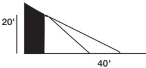
Solution: Mounting at 6 feet to 12 feet allows maximum range.
