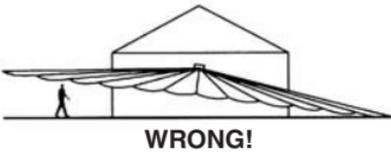
Solution: Position sensor exactly level from side to side.
