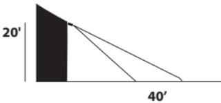
**Solution:** Mounting 6-12ft allows maximum range
