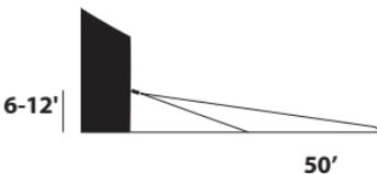
3. Check that movement is not directly towards sensor. Sensor will see movement across its pattern more quickly. To fix, move sensor.
