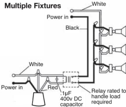
Multiple fixtures may be wired to a single sensor.
