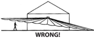
**Solution:** Position sensor exactly level from side to side.
