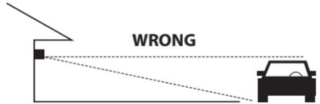
**Solution:** A 20ft safety zone and reduced sensitivity are recommended to avoid activation from passing cars.
