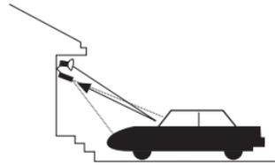
**Solution:** Aim sensor away from reflective objects or move the objects lower and reduce sensitivity.
