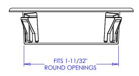
SUITABLE FOR 2"X3" AND 2"X4" METAL STUDS WITH PUNCHED HOLE DIAMETERS OF 1-11/32"
