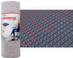
NUHEAT MEMBRANE by Progress Profiles is a tile underlayment and uncoupling system that is specifically designed to embed and hold the industry-leading Nuheat Cable floor heating system. The low profile of the Membrane reduces the stress caused by differential movement between the tile layer and the substrate which can lead to tile cracking.
