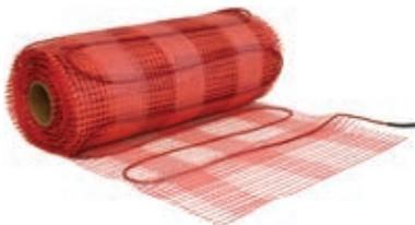
The Nuheat Mesh system is a heating cable woven into an adhesive-backed fiberglass mesh with patented mesh bands to hold the heating cable in place. The modifiable solution is simple to roll-out and can be customized to fit any room shape.
