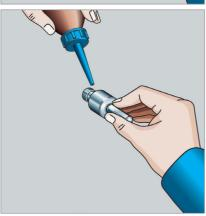
Apply lubricant to adapter's finepitch thread for every change. This makes it easier to release the adapter later on.
