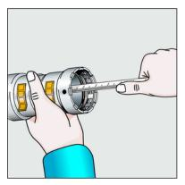
Measure insertion depth in the connector.
