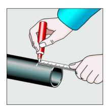
Mark the insertion depth on the pipe.
