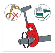
Cut the pipe using a pipe cutter, angle grinder or fine-toothed hacksaw. Do not use a flame cutter
