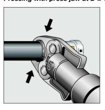
■ Insert the press jaw (≤ D 1) into the press machine and push the retaining bolt in as far as it will go.
