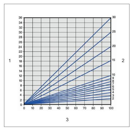
Fig. 3: Length expansion steel pipes
