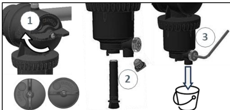
Bypass and Blowdown Service
