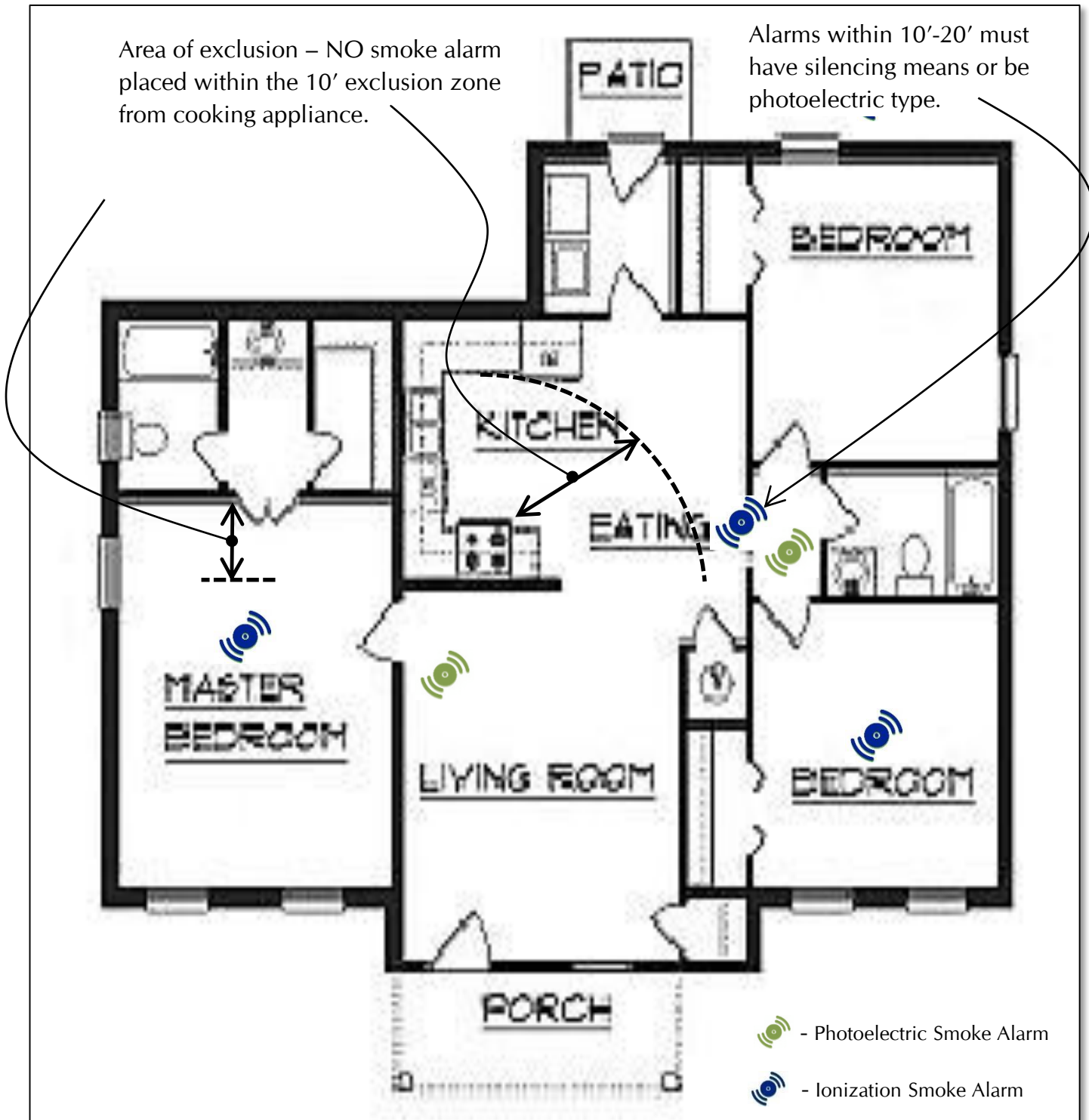
Figure 2: Alarm Placement in a Small Home
